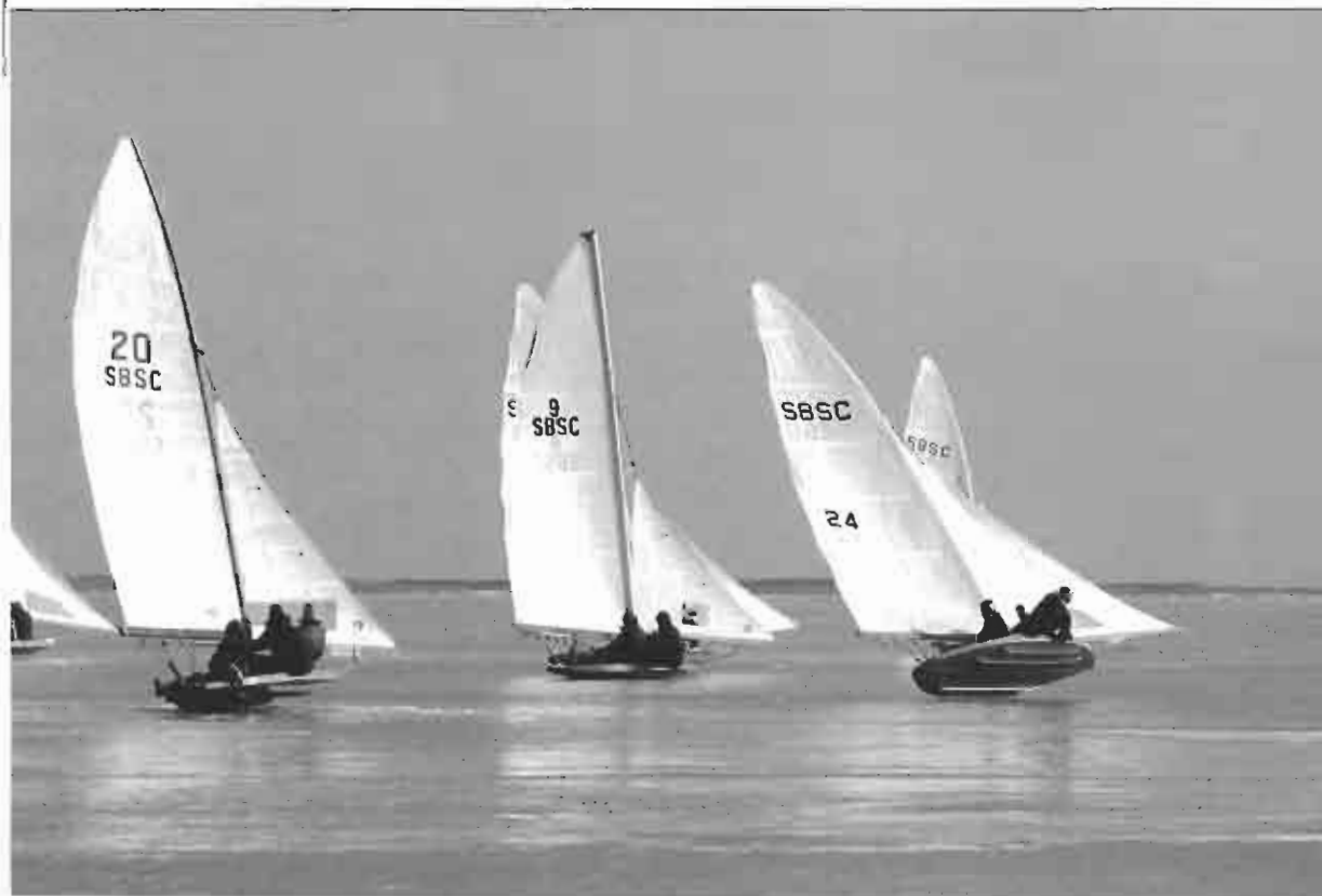
Dick Richardson (#20), Bob Hermus (#9), Robin Paris (#24), and other members of the fleet scoot toward the finish line. Paris's boat has a Harless-style cane-mast airfoil rig. Richardson's and Hermus's are fully battened marconi rigs on boats designed by Bob's grandfather, Frank Hermus, in the 1940s.
