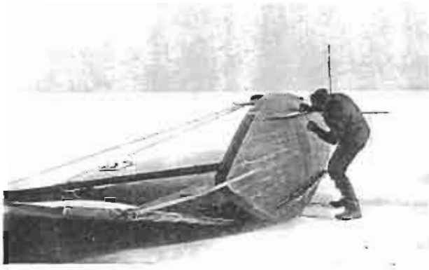
An important operation on a "Scooter" — sharpening up the runners
